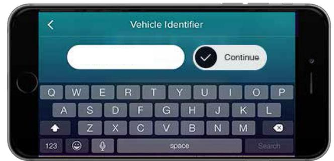
8. Adjust your registration plate to view in the scanning box area and press '**Auto Detect Plate**' (UK only). Alternatively, manually enter your registration in '**Manually Enter**' (Non UK) option given and press '**Continue**'. Alternatively, the scanning box area can also read a barcoded VIN.
