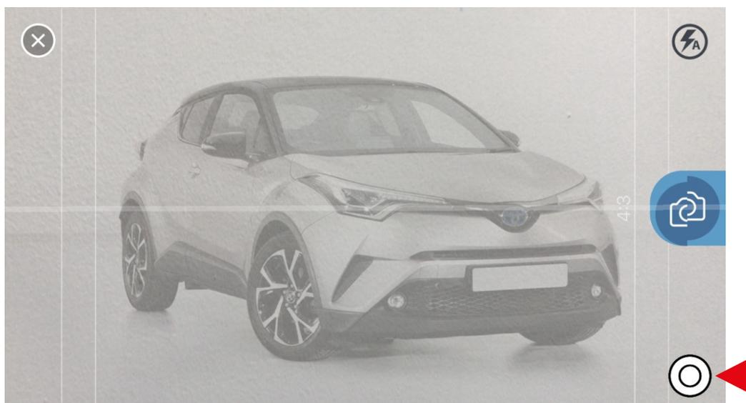
The Split button feature will ensure you have the correct angle every time. You need to ensure you hold the device at the right angle and the app will help you do just that. When the device is at the wrong angle the button with the camera on will turn red and split in half, sliding up and down the screen on the right hand side, as can be seen in the screenshot below.
